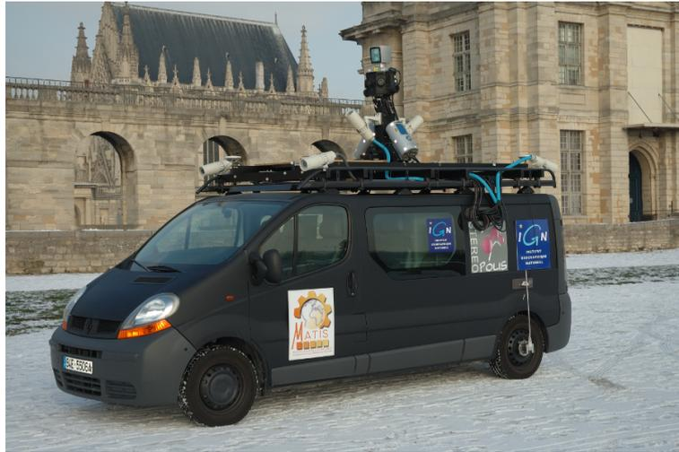
**Figure 1** : The STEREOPOLIS II mobile mapping system.
