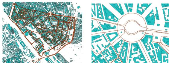
**Figure 10** : Footprint of the survey acquired on 12th district of Paris in April 2008 for the iTOWNS ANR project. One point in red corresponds to one image node. In blue, the IGN building database is displayed. **Left**: Overview of the area. **Right**: Focus on a roundabout.
